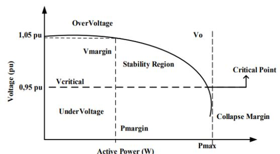
**Figure 1** P-V Curve Graph (Active Power vs. Voltage)
