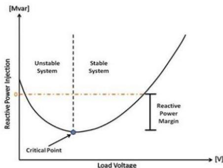
**Figure 2** Q-V Curve (Reactive Power vs. Voltage)
