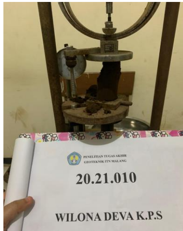
Gambar 4.14 Pengujian Unconfined Compressive Strength
