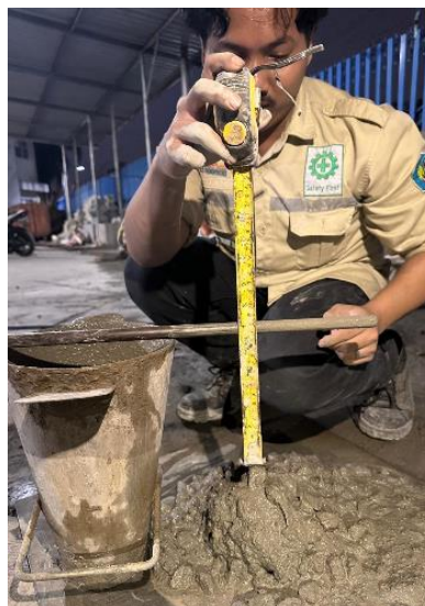
Gambar 4. 32 Slump Test Variasi 0,1% Sumber:( Hasil Penelitian)
