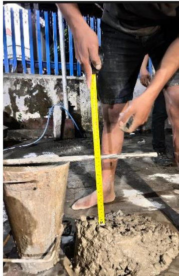
Gambar 4. 31 Slump Test Variasi 0% Sumber:( Hasil Penelitian)
