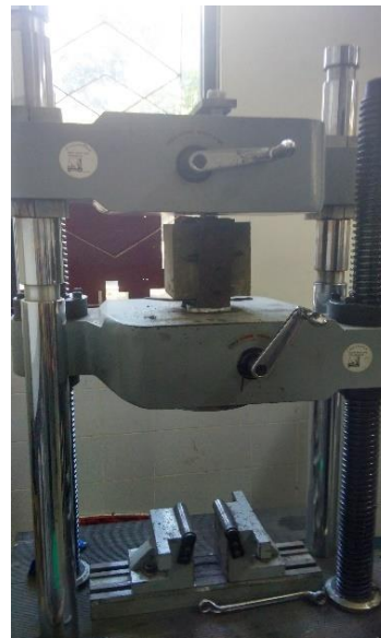
Alat uji tarik Universal Testing Machine
