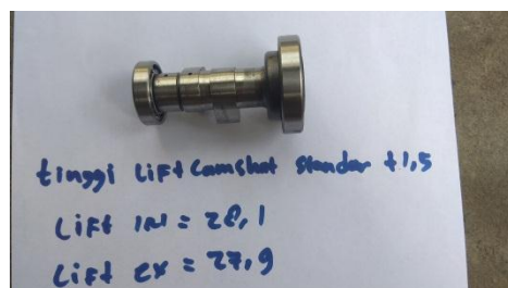
Gambar 3.14 camshaft standar penambahan tinggi lift 1,5mm (sumber gambar pribadi)
