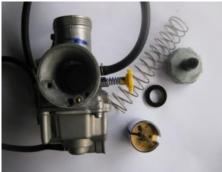
Gambar 4.5 Karburator rx king ukuran 26mm
