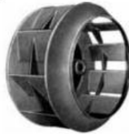
Gambar 2.11 Backward inclined fan (Sumber : US DOE, 1989)
