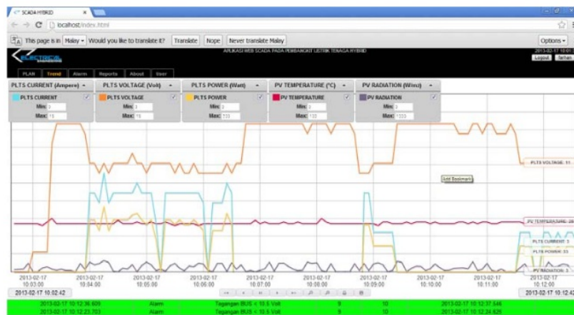
Figure 8. Trending display of solar power system
