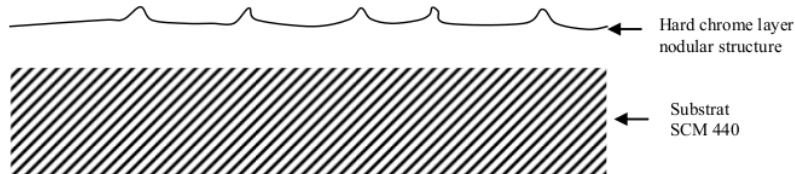
Figure 2 The picture of nodular structure illustration of the chrome surface layer
