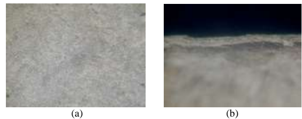
Fig 3. AISI 4140 Microstructure (250x) a) before, b) after nitriding
