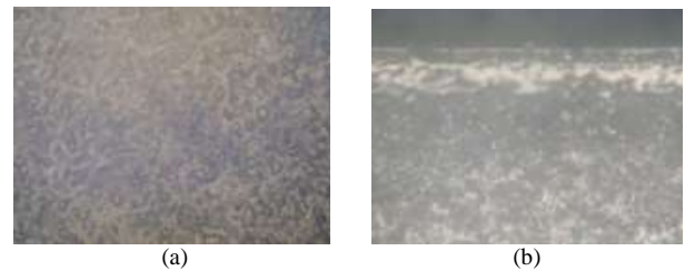
Fig 2. AISI 4340 Microstructure (250x) a) before, b) after nitriding
