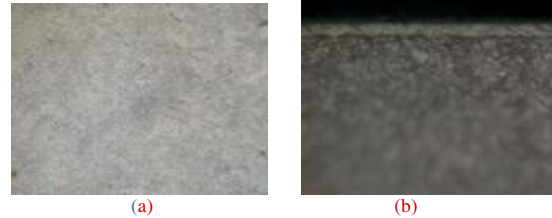
Fig 1. AISI P20 Microstructure (250x) a) before, b) after nitriding
