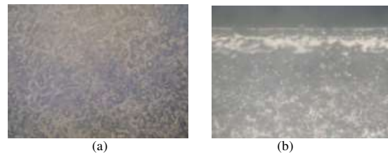
Fig 2. AISI 4340 Microstructure (250x) a) before, b) after nitriding
