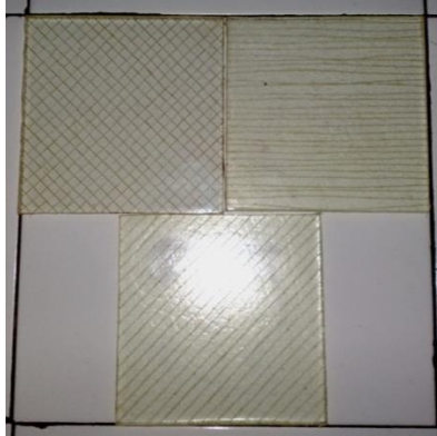
Figure 7. Fiber orientation wall tile product
