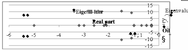
Fig. 4. Eigenvalues of best compromise solution of UPFC placement for IEEE 30-bus system.
