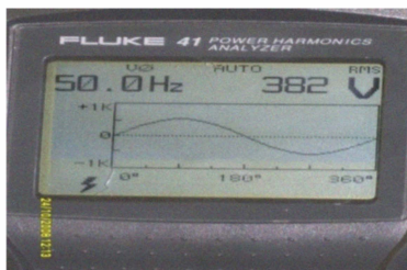
Figure 11. Fluke Power Analyzer under Measurement.
