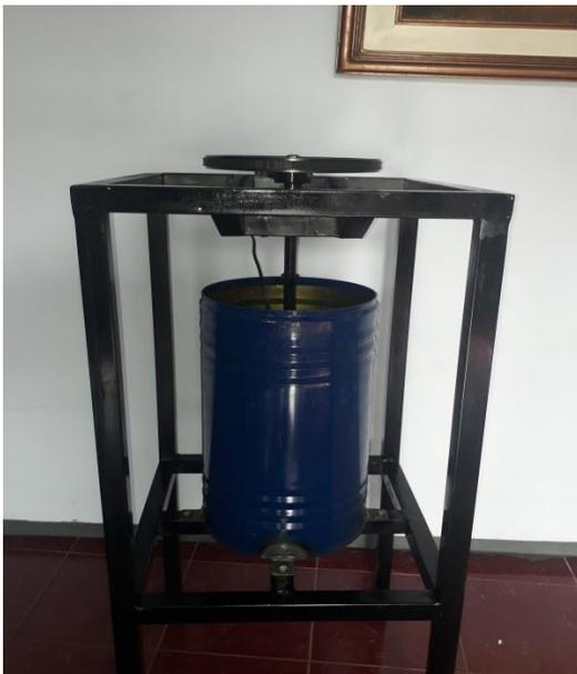
Gambar 7 Desain rancangan alat *mixing* sabun cair
