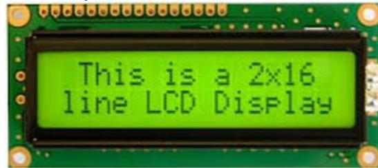
Gambar 2.3 LCD Display
