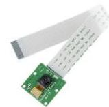
Gambar 2.16 Camera Raspberry Pi Module v1
