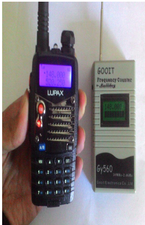
Gambar 4. 2 Pengujian Transmitter HT 148.000 Mhz
