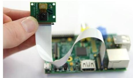
Gambar 6 Raspberry Pi Cam
