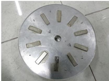
Gambar 3.3 Rotor Magnet Permanen
