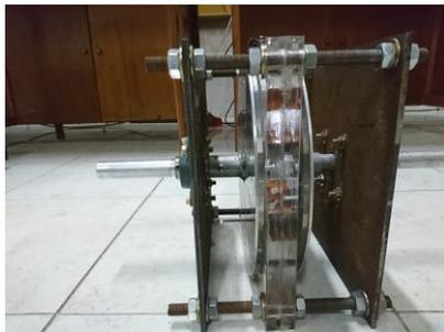
Gambar 3.6 Generator magnet permanen
