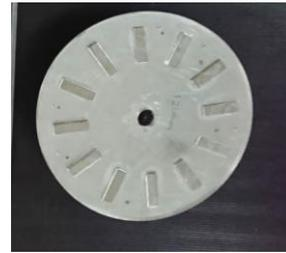
Gambar 3.5 Rotor Generator Magnet Permanen
