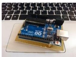
**Gambar 2.5** Mikrokontroler Arduino Uno R3
