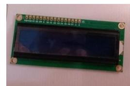
**Gambar 2.16** LCD 16 x 2
