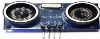
Gambar 2.7 Sensor Ultrasonic
