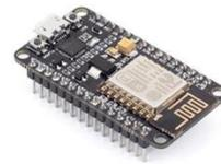
Gambar 2.2 Modul Wifi NodeMCU
