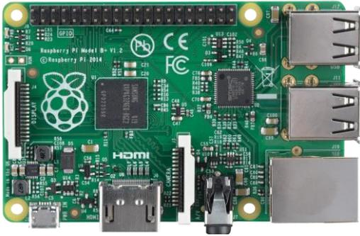
Gambar 2.1 Raspberry Pi Board
