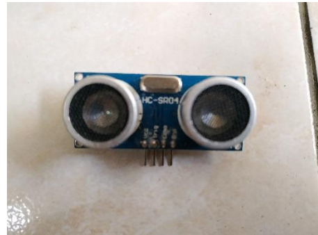
Gambar 2.10 Sensor Ultrasonik HC-SR 04
