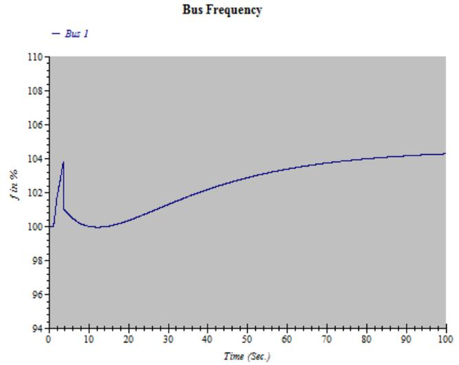
Figure 2: Frequency response during 3 phase short circuit (t=1 s)
