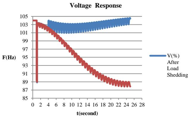
Figure 7: Voltage response before and after load shedding
