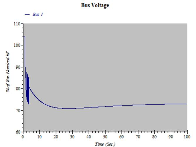
Figure 3: Voltage response during 3 phase short circuit (t=1 s)
