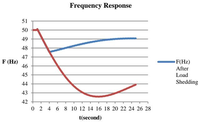
Figure 6: Frequency response before and after load shedding
