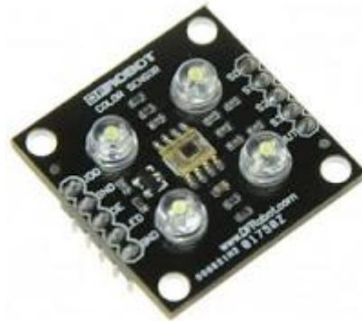
Gambar 2.2 Sensor Warna TCS3200
