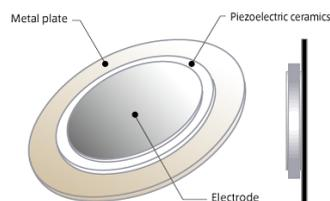
Gambar 2.2.2 Sensor Piezoelectric
