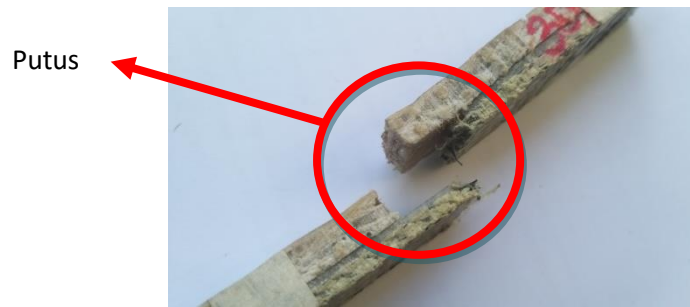
Gambar 6. Hasil uji tarik specimen karet silikon 30%
