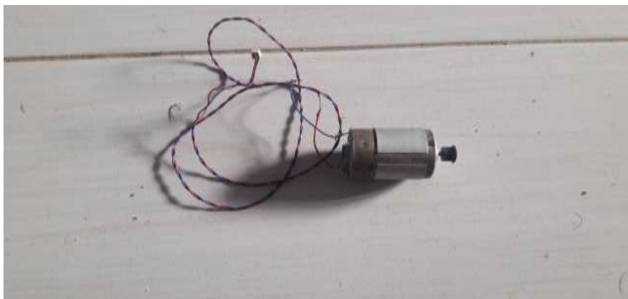
III-1 8 Generator DC 12Volt
