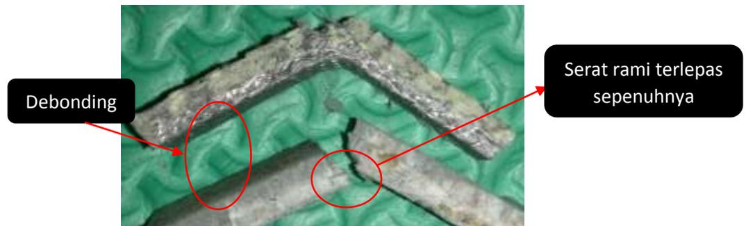
Gambar 4.4 Patahan Spesimen Uji Impact Persentase 30% Karet
