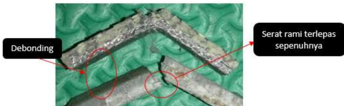
Gambar 8 Patahan Spesimen Uji Impact Persentase 30% Karet
