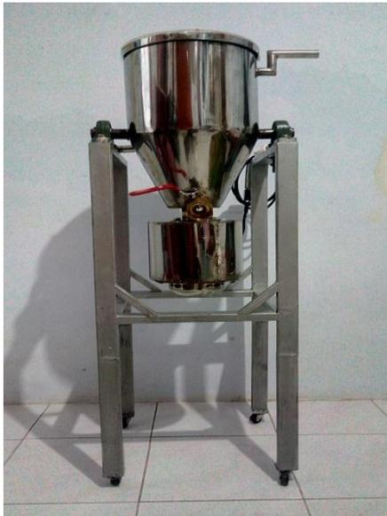
Gambar 4.8 Desain rancangan alat *mixing* sabun cair
