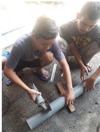
Proses Pemotongan Pipa PVC 3 inch
