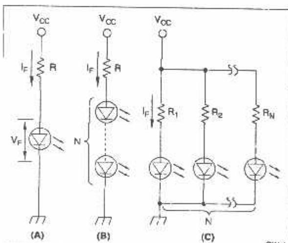
Figure 1. Driving Circuit of Light-Emitting Diode (LED)
