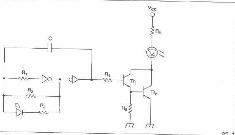
Figure 14. Pulse Driving Circuit using CMOS Logic IC
