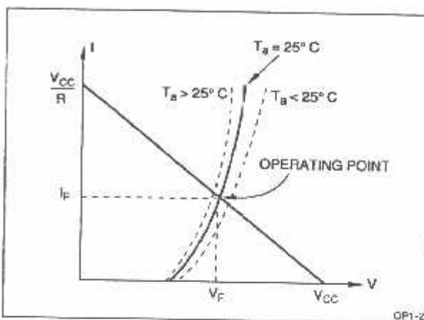
Figure 2. Current versus Voltage of Light-Emitting Diode (LED)
