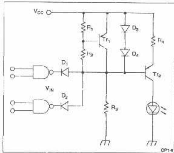
Figure 8. Connection with the TTL Logic Circuit (3)
