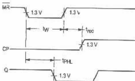
Figure 2. Master Reset Pulse Width,
