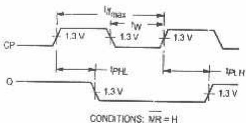
Figure 1. Clock to Output Delays
