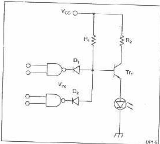
Figure 6. Connection with the TTL Logic Circuit (2)
