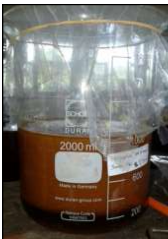
Figure 5. Chemical delignification process
