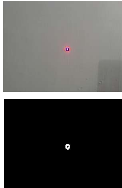
Fig. 3. Detected laser spot on white background.
