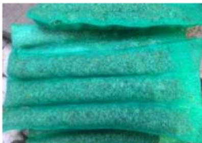
Fig. 13. Packed concrete sand (to be put into the filtering pipe)
