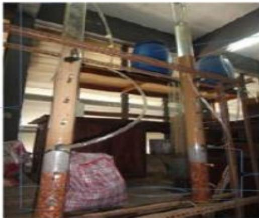
**Gambar 5.** Desain filter pasir
