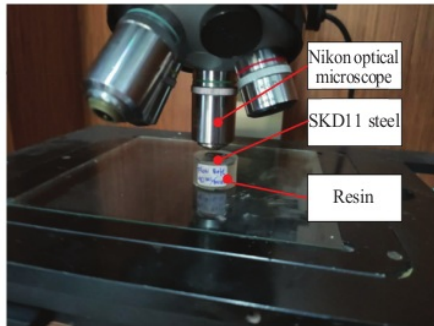
Fig. 4. Testing the thickness of the carbon thin film on the sample with the Nikon Type 59520 Optical Microscope
