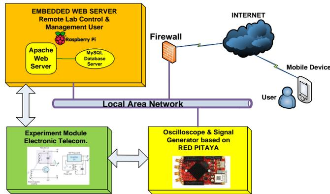
Fig. 2. Design Remote Laboratory
