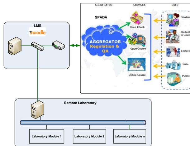
Fig. 1. Integration of SPADA, LMS and Remote Lab
