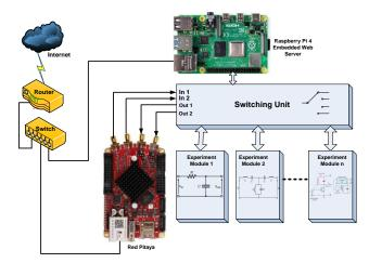
Red Pitaya instrumentation unit. The switching unit is controlled by the Raspberry Pi 4 according to the commands given by the user remotely via the web interface.
