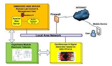
Fig. 2. Design Remote Laboratory
