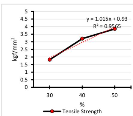
Gambar 3. Effect of Fraksi Massa on Tensile Strength
