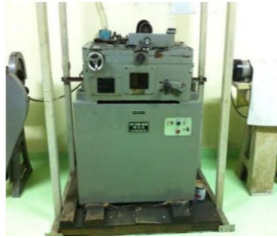
Figure 2. Wear testing ogoshi method
