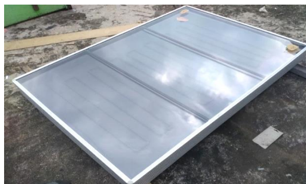
b. a fabricated solar collector design
