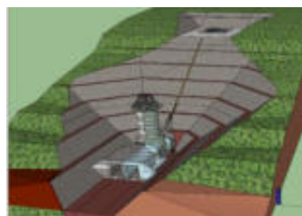
Figure 8 inlet and shaft construction
