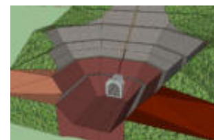
Figure 9 Outlet construction with channel normalization to the river
