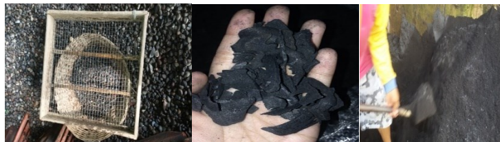
Figure 1. Materials for filter (Gravel 12.5 mm, 2 mm Charcoal and 2 mm Sand)
