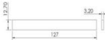
Figure 3: Bending test specimen dimension [9]
