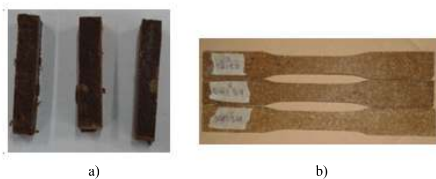
Fig 2. a) Composite and b) impact test specimen
