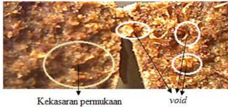
Fig 3. Macro Composite Photo of Coconut Powder with Polyester Matrix
