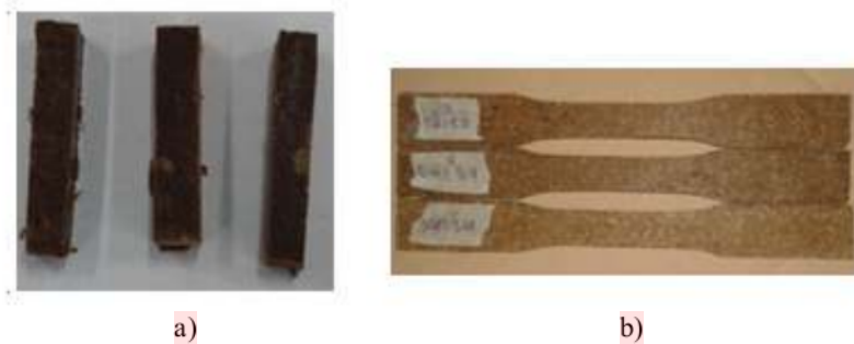
Fig 2. a) Composite and b) impact test specimen
